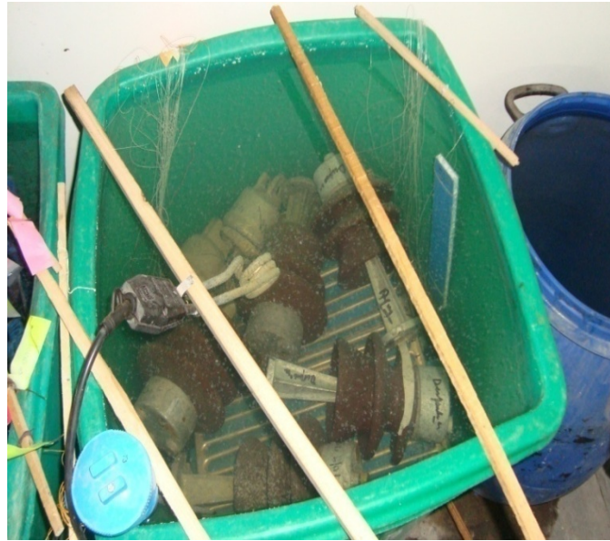
Figure 1 Heating element and RTD sensor in a tank.
