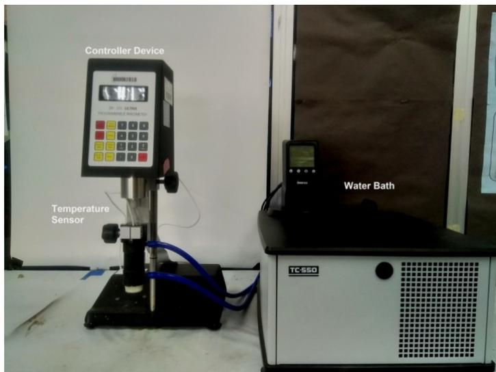
**Figure 3** Brookfield LVDV III Ultra Rheometer for the measurement of dynamic viscosity (from left: temperature sensor, controller device and water bath).
