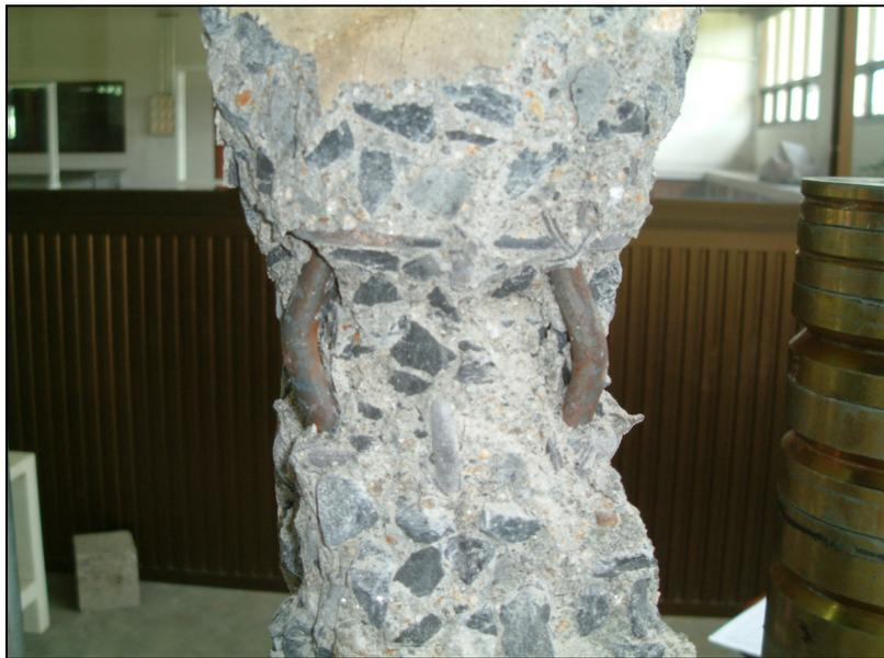
**Figure 3** Failure in a column specimen.
