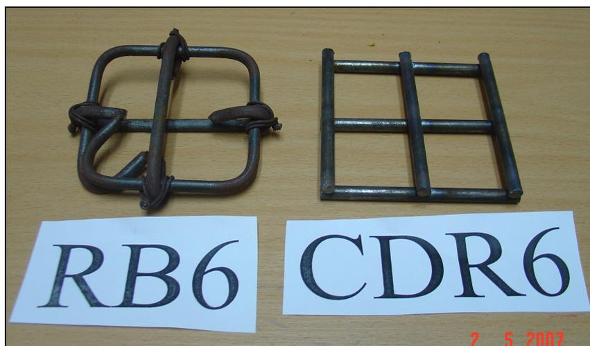
**Figure 1** Two types of transverse reinforcement of column specimens.
