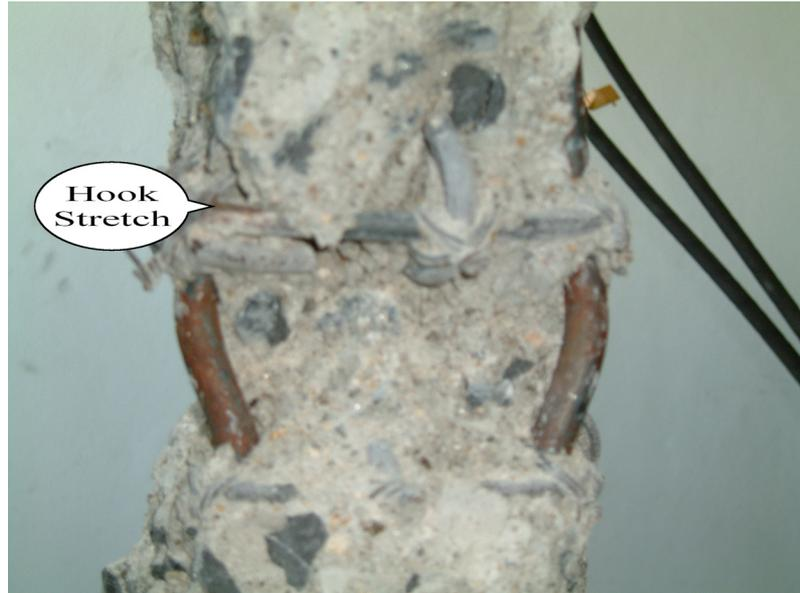
**Figure 5** Hook stretch in conventional tie caused failure of specimen RB6(5.0).
