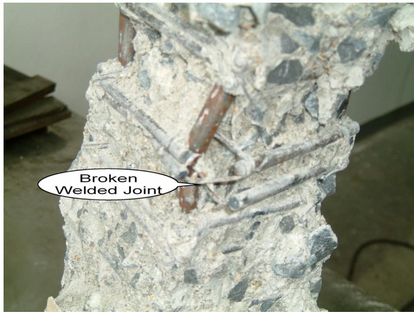
**Figure 4** Breaking at a welded joint of WWF caused failure of specimen CDR 6(2.5).
