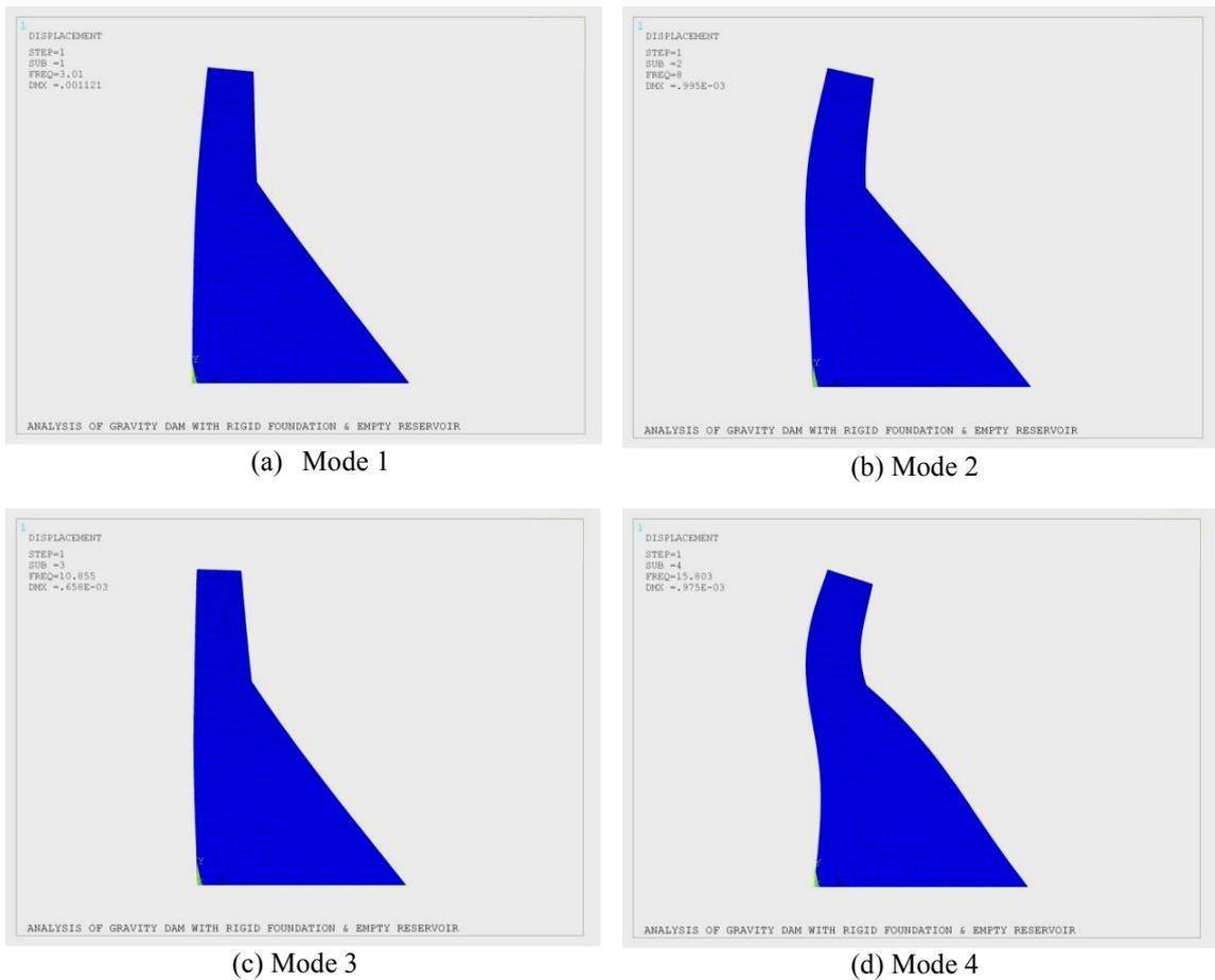
**Figure 7** The first 4 mode shape of the dam for case 1 [23].
