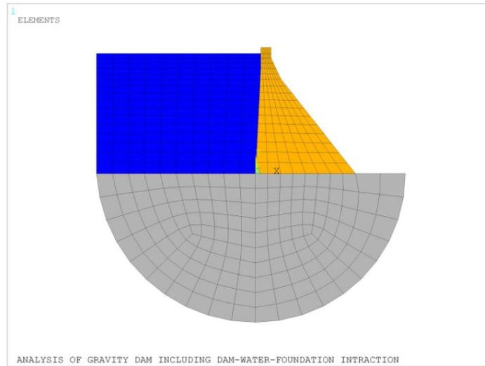
**Figure 4** Finite-element model of Pine Flat dam-water-foundation rock system [23].
