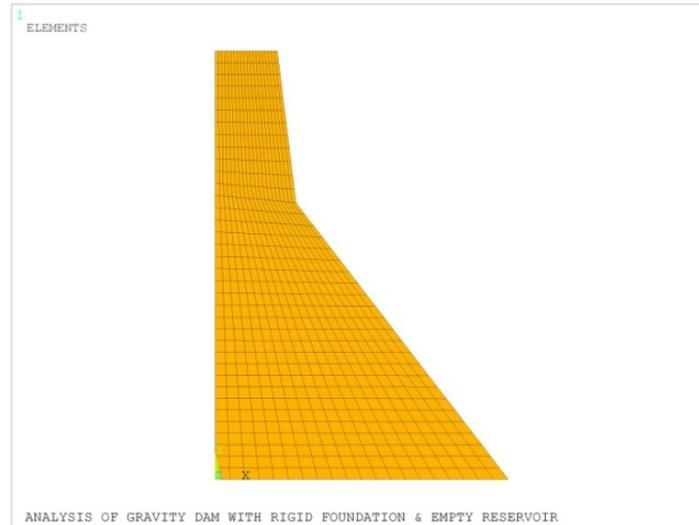
**Figure 6** Finite-element model of Koyna dam (dam with empty reservoir and rigid foundation) [23].
