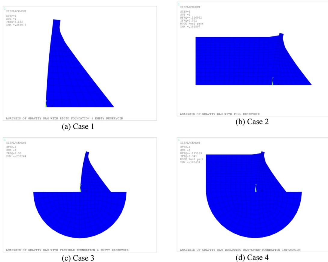
**Figure 5** The first mode shape of the dam for different cases [23].
