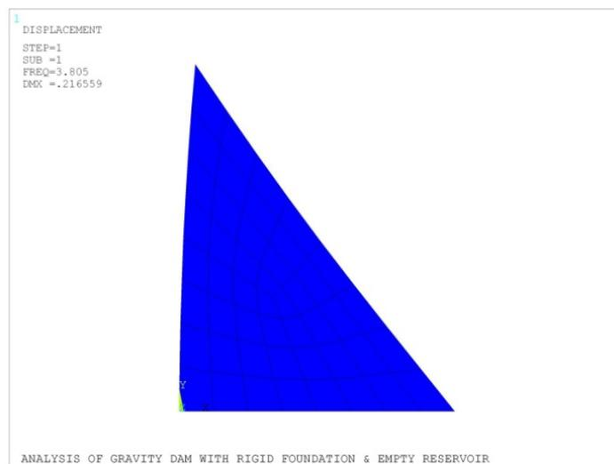
**Figure 8** The first mode shape of the dam for case 1 [23].
