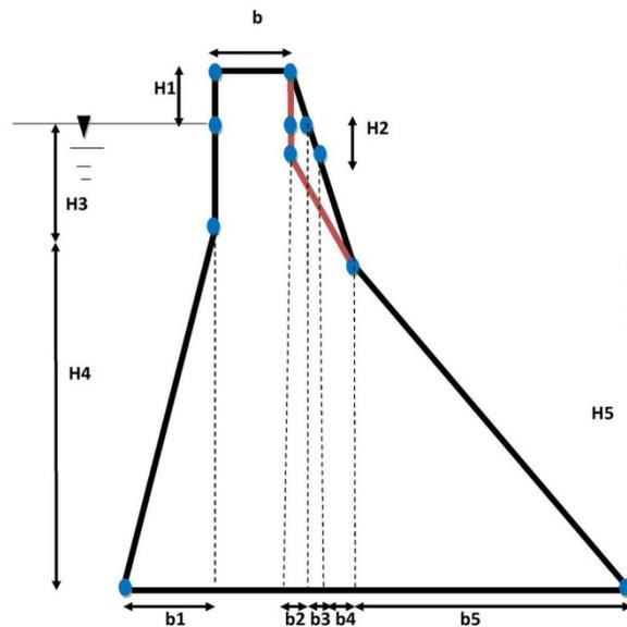
**Figure 2** The geometric variables of the gravity dam [23].
