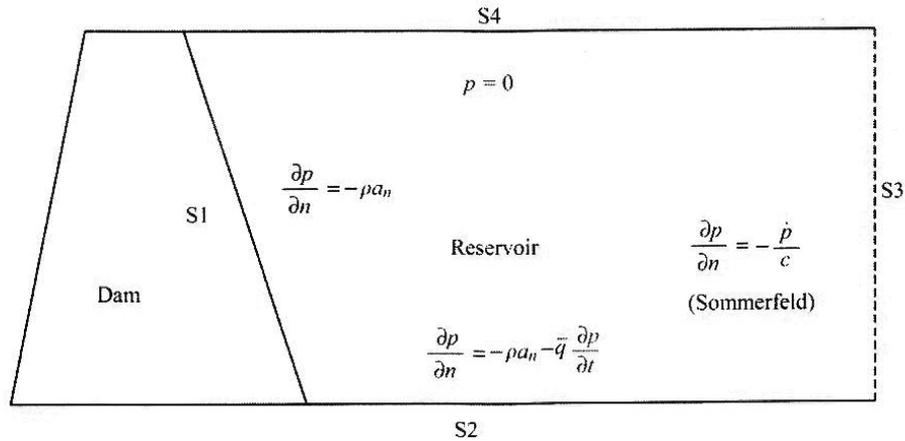
**Figure 1** The boundary conditions of the fluid domain [20].
