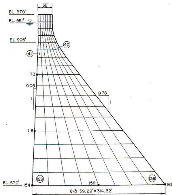
**Figure 3** Dimensions of the tallest monolith of Pine Flat dam [24,25].
