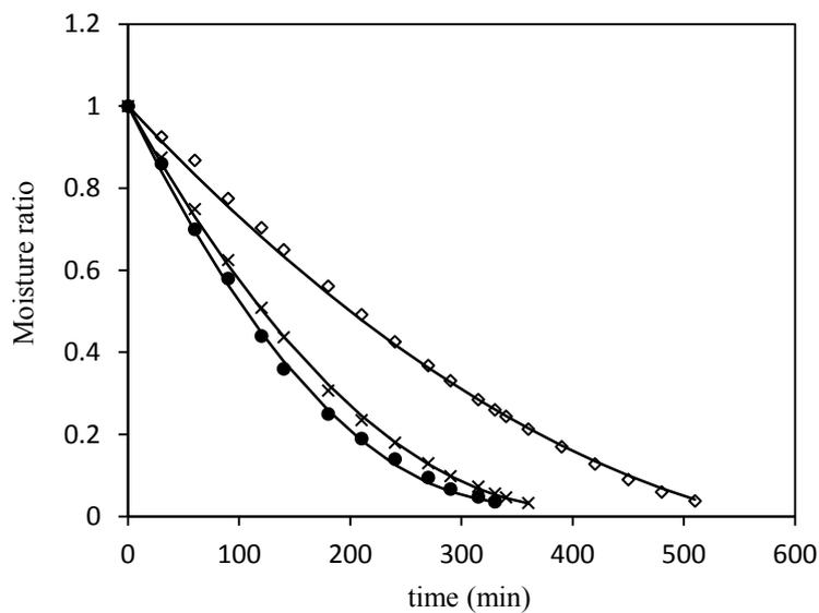
**Figure 4** Comparison between experimental data and best fit of Wang and Singh model at different temperatures: ( $\diamond$ ) 55 °C, ( $\times$ ) 60 °C, ( $\bullet$ ) 65 °C, (—) prediction.
