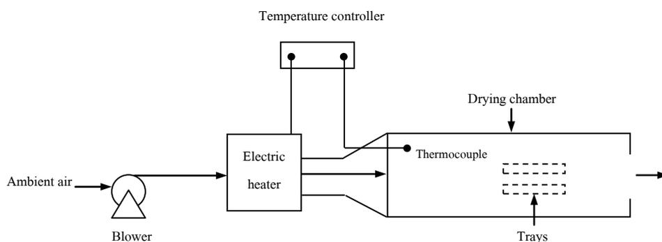
**Figure 1** Schematic diagram of hot air dryer.
