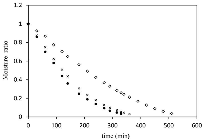
**Figure 2** Drying curves of chilies at different temperatures: (◇) 55 °C, (×) 60 °C, (●) 65 °C.
