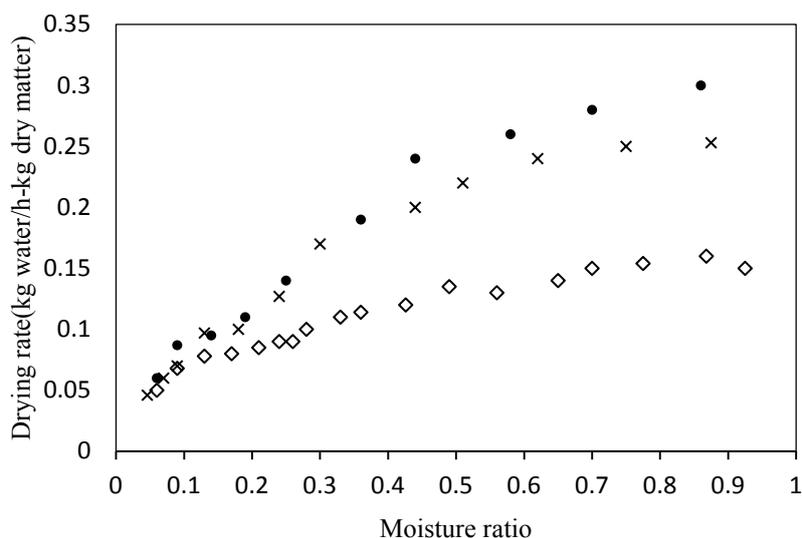
**Figure 3** Variation of drying rate with moisture ratio at different temperatures: (◇) 55 °C, (×) 60 °C, (●) 65 °C.
