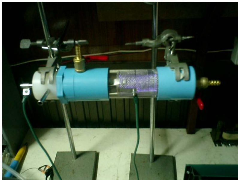
Figure 5 Picture of ozoniser tube when the discharge occurred and ozone is produced.
