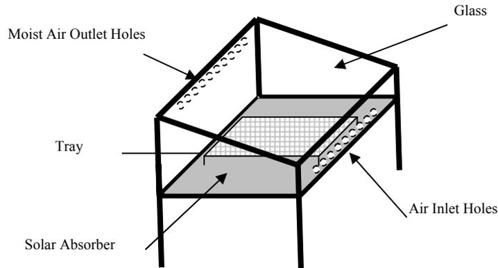
**Figure 1** Features of the box solar dryer.
