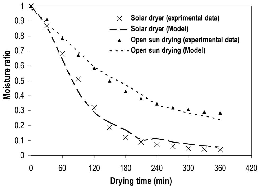
**Figure 6** Comparison of the moisture ratio between experimental data and calculated values according to the Henderson & Pabis model.
