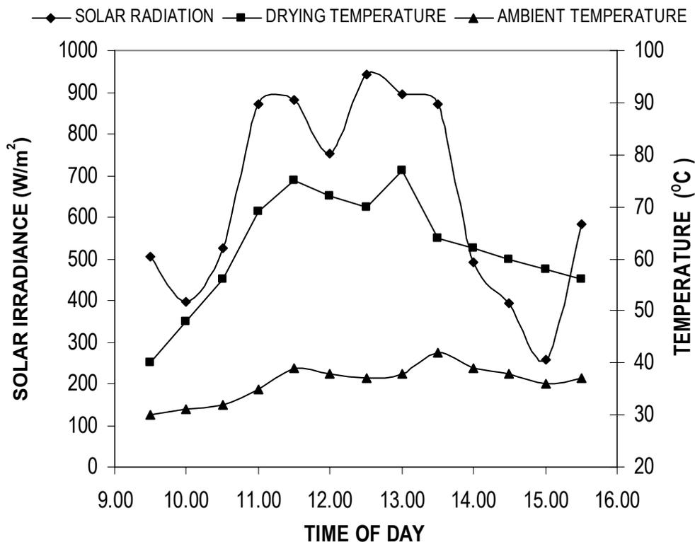
**Figure 2** Flux density of solar radiation and temperature profiles during a typical day.
