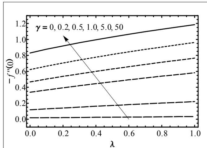
**Figure 5** Variation of the skin friction  $-f''(0)$  for different values of  $\lambda$  and  $\gamma$ .
