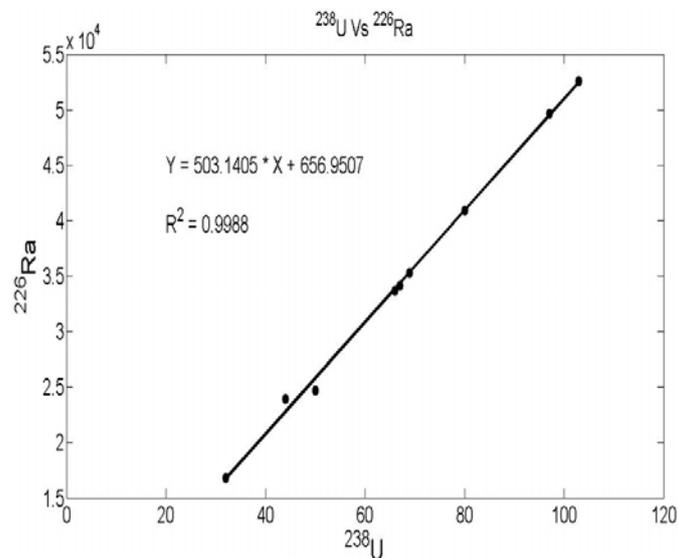
**Figure 8** The correlation between  $^{238}\text{U}$  and  $^{226}\text{Ra}$  concentration in oil well-cores.
