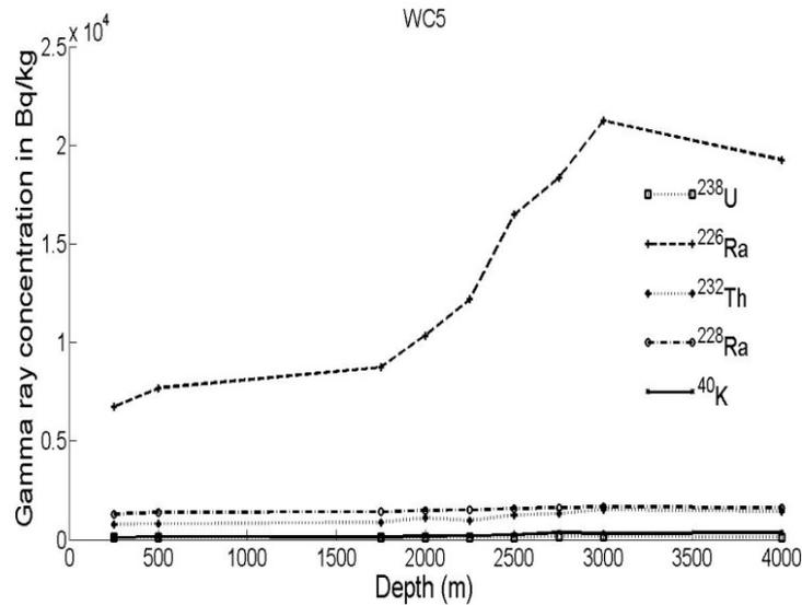
**Figure 7** Gamma radioactivity concentration as a function of well core depth (WC5).
