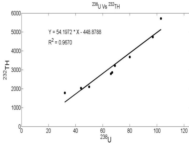
**Figure 10** The correlation between  $^{238}\text{U}$  and  $^{232}\text{Th}$  concentration in oil well-cores.
