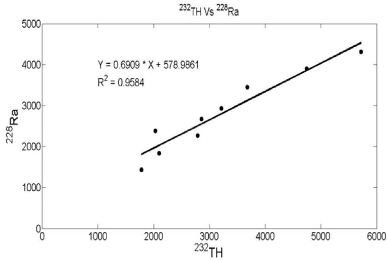
**Figure 9** The correlation between  $^{238}\text{Ra}$  and  $^{232}\text{Th}$  concentration in oil well-cores.
