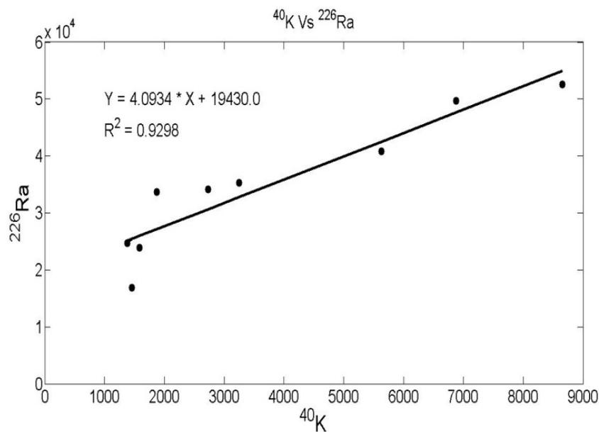
**Figure 12** The correlation between  $^{226}\text{Ra}$  and  $^{40}\text{K}$  concentration in oil well-cores.
