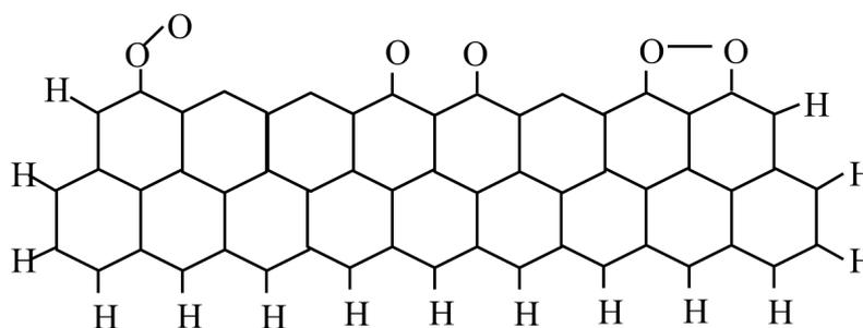
**Figure 4** Different forms of oxygen adsorption at the edge of the activated carbon layer (Adapted from Truong *et al.* [51])
