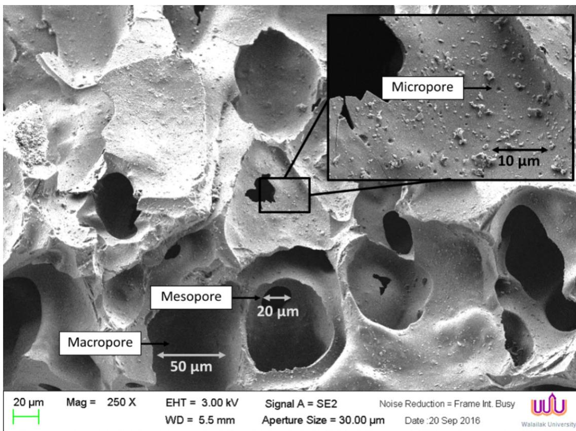
**Figure 2** Pore structure of stream-activated granular bituminous coal-based activated carbon.
