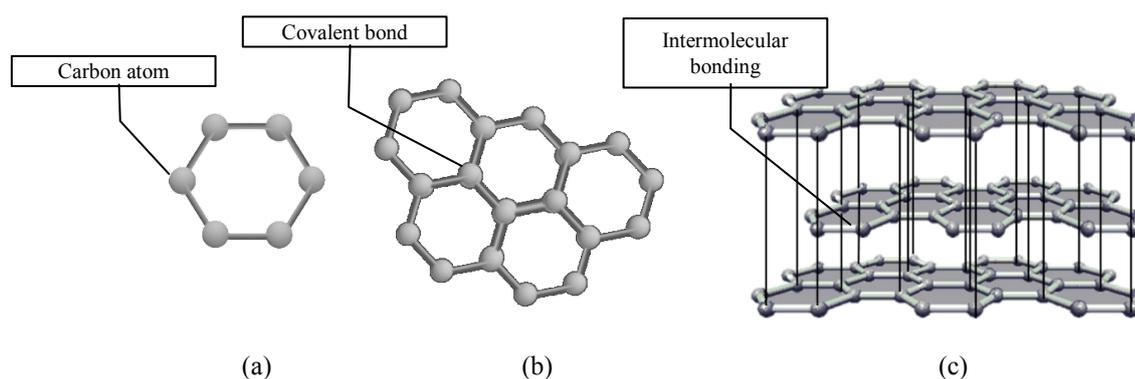
**Figure 1** Hexagonal carbon atom (a), microcrystalline carbon layer (b), and activated carbon structure (c).
