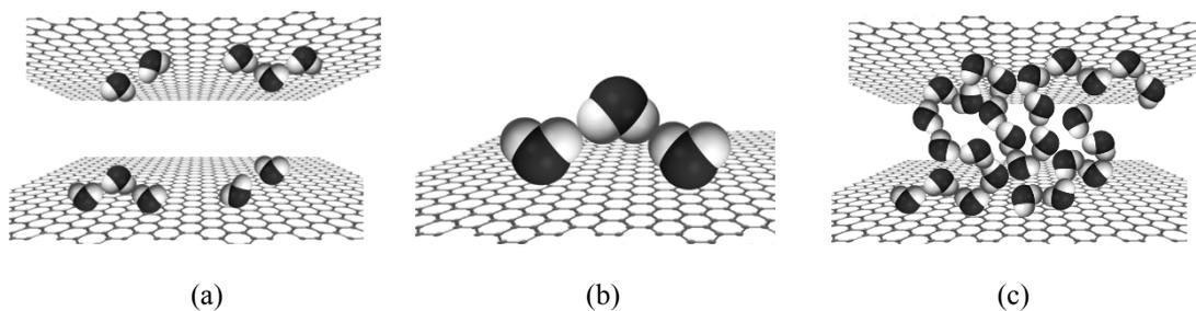
**Figure 5** The configuration form of water molecule on activated carbon pore surface at low pressure (a) at the nucleation site (b) and at high pressure (c) (Adapted from Müller *et al.* [68]).
