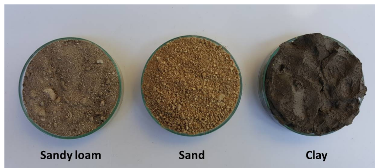
Figure 1 Physical characteristics of different soil substrates in simulated earthen pond conditions during the culture period: sandy loam (75.1 - 80.9 % sand, 6.7 - 12.8 % silt and 12.0 - 16.0 % clay), sand (92.9 - 95.1 % sand, 2.7 - 4.8 % silt and 2.0 - 2.2 % clay), and clay (17.2 - 22.9 % sand, 2.7 - 6.7 % silt and 72.2 - 78.0 % clay).
