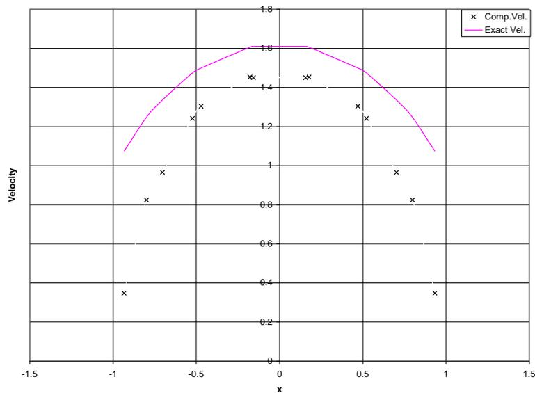
**Figure 6** Comparison of computed and analytical velocity distributions over the surface of the sphere using 96 boundary elements.
