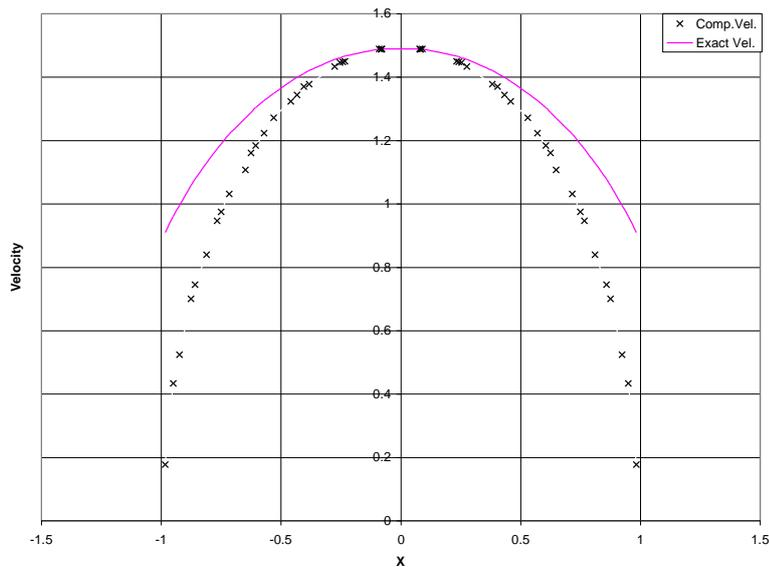
**Figure 7** Comparison of computed and analytical velocity distributions over the surface of the sphere using 384 boundary elements.
