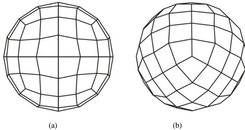
**Figure 4** Discretization of sphere into 96 boundary elements. The point of observation is (a) on the z-axis; (b) at  $45^\circ$  to all axes.
