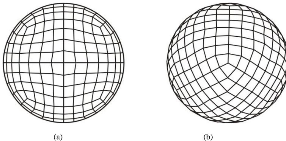
**Figure 5** Discretization of sphere into 384 boundary elements. The point of observation is (a) on the z-axis; (b) at  $45^\circ$  to all axes.
