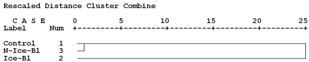
**Figure 5** Cluster analysis of poplar specimens based on impact strength, MOR, MOE, and compression strength parallel to the grain values.
