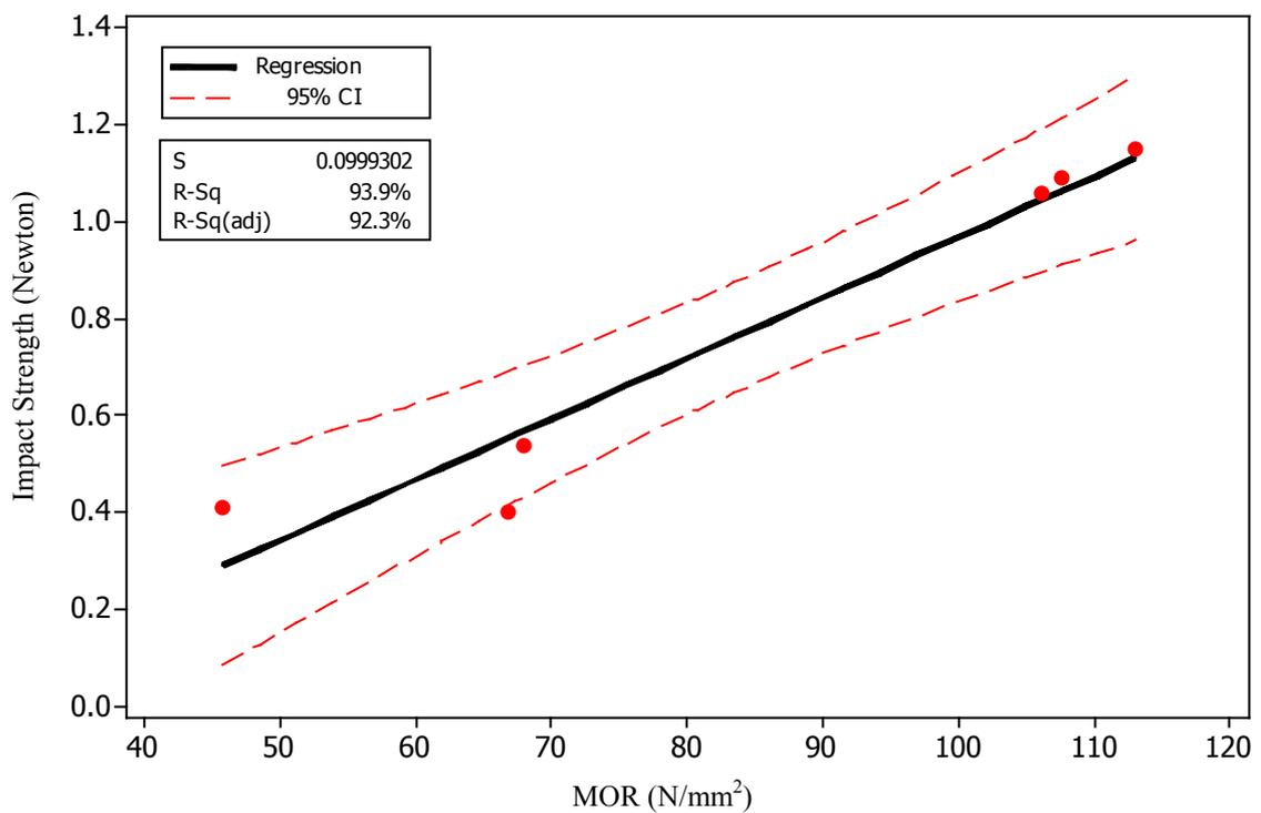
**Figure 7** Fitted-line plot between impact strength versus modulus of rupture (MOR).
