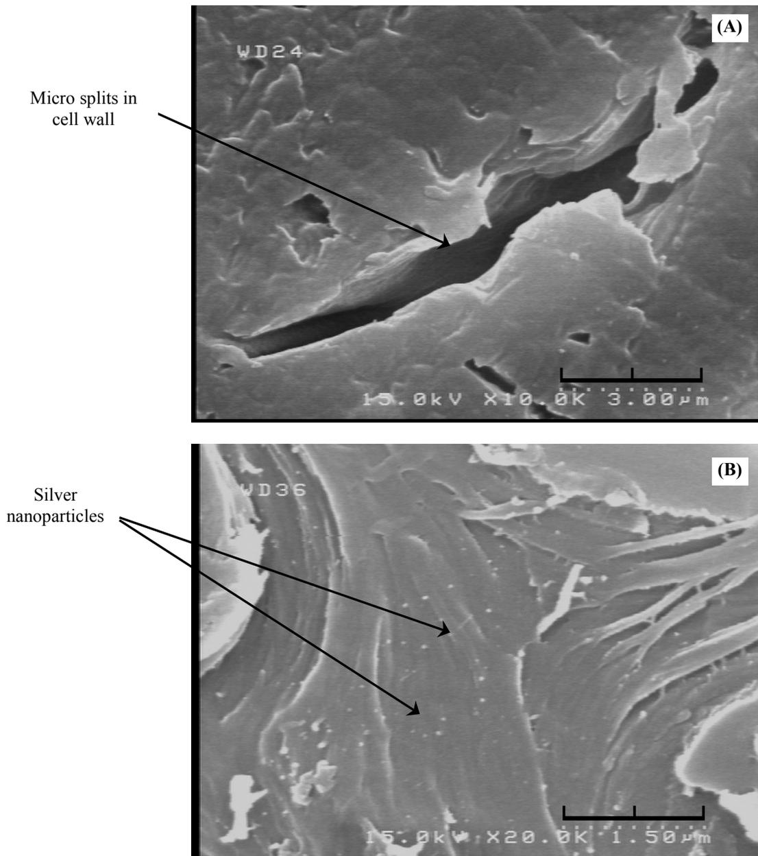
**Figure 1** (a) Fissures and splits (↓) occurred in cell wall due to extreme cold shock caused by ice-blast treatment on beech specimen [8,17]; (b) silver nanoparticles (↓) spread all over the cell wall.
