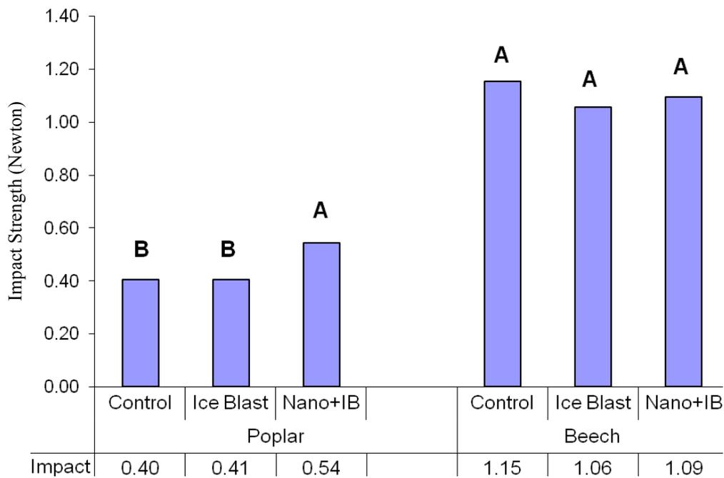
**Figure 2** Impact bending strength values of 3 groups of control, ice-blasted, and nanosilver impregnated ice-blasted poplar and beech specimens (Newton) (IB = Ice-Blasted) (Letters on each column represent Duncan multiple range groupings at 95 % level of confidence).
