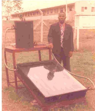
Figure 3 The experimental set-up of the solar water heating system.
