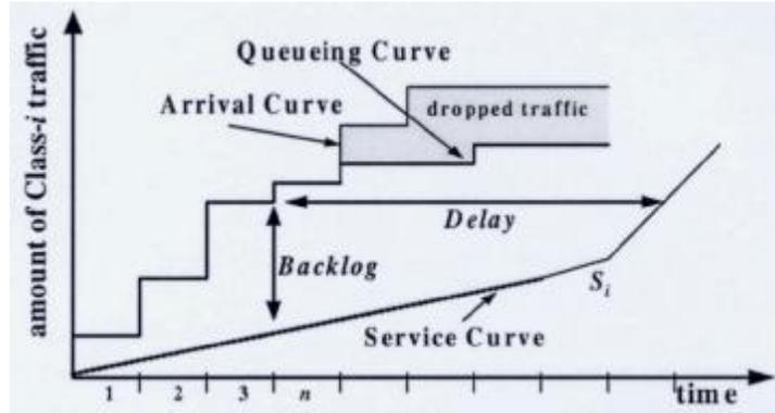
**Figure 2.** Traffic curves and system performance parameters.
