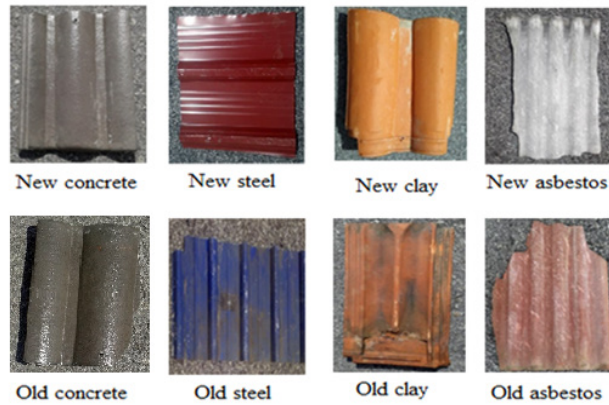
Figure 3 Samples of the roof materials (different types and conditions).
