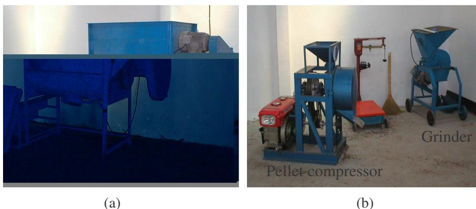
**Figure 1** (a) the horizontal fertilizer mixer, (b) the organic fertilizer grinder and the pellet compressor.
