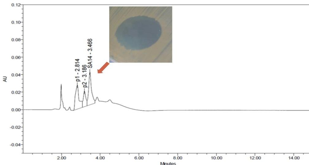
**Figure 5** RP-HPLC elution profile of antimicrobial peptide purification.
