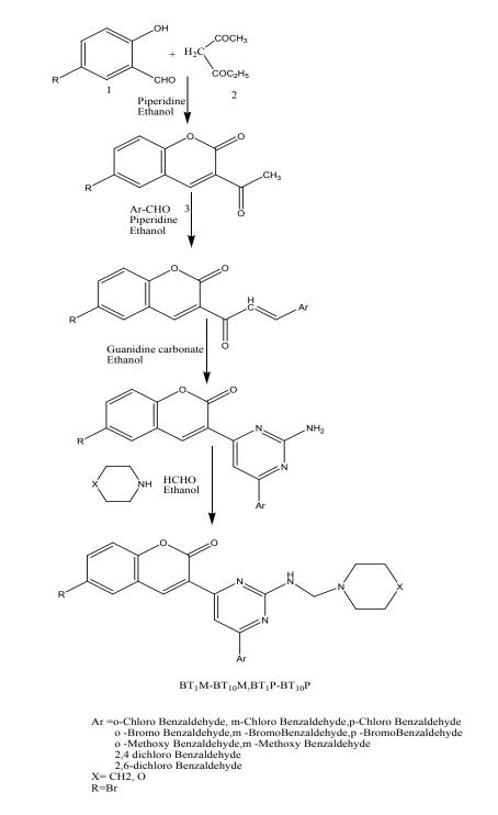
Scheme 1 Schematic diagrams for the synthesis of pyrimidine derivatives (BT<sub>1</sub>M-BT<sub>10</sub>M, BT<sub>1</sub>P-BT<sub>10</sub>P).
