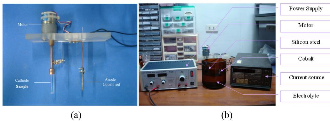
**Figure 1** Photographs of (a) electrodes and (b) an electrodeposition system.
