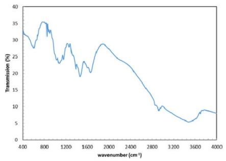
Figure 4 FTIR Spectra of chitosan powder.
