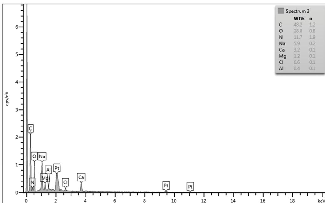
**Figure 2** SEM-EDX elemental composition analysis of chitosan.
