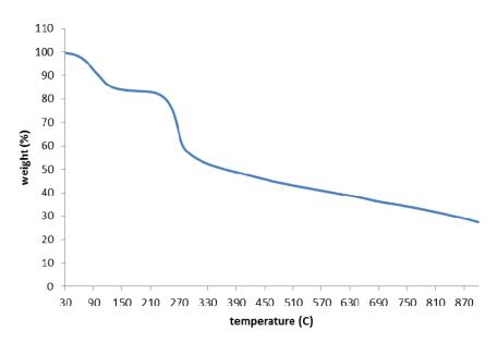
Figure 5 TGA Curves of thermal degradation of extracted chitosan powder.
