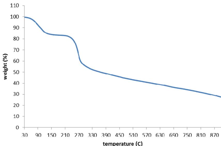
**Figure 5** TGA Curves of thermal degradation of extracted chitosan powder.
