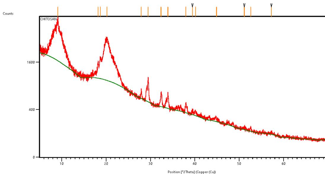
**Figure 3** X-Ray Diffraction pattern of chitosan powder.
