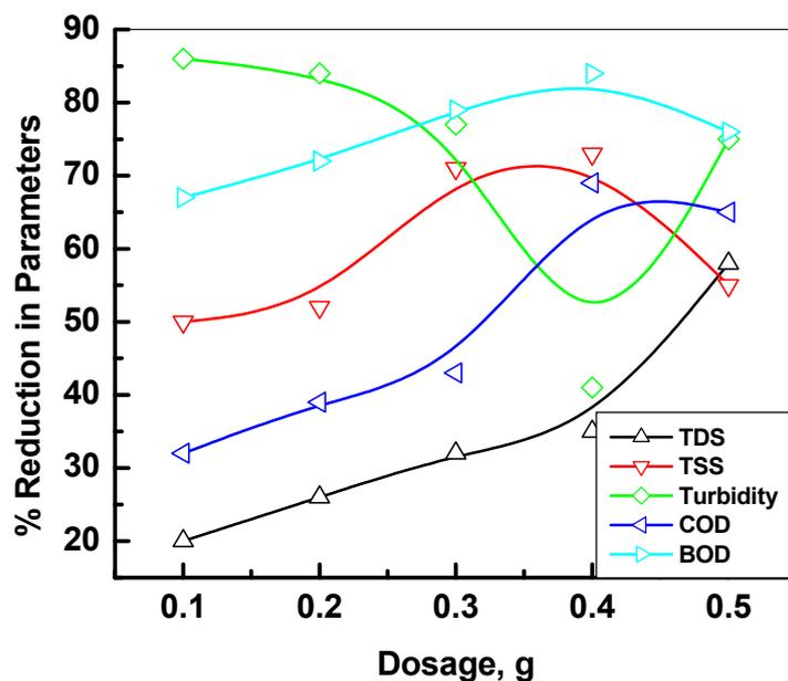
**Figure 8** Effect of variation of dosage of chitosan with parameter reductions.
