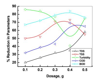
Figure 8 Effect of variation of dosage of chitosan with parameter reductions.
