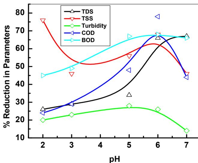
**Figure 6** Effect of variation of refinery effluent solution pH with parameter reductions.
