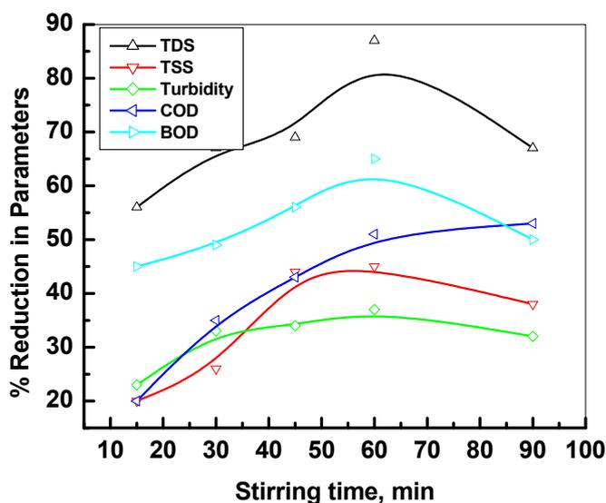
**Figure 7** Effect of variation of mixing time with parameter reductions.
