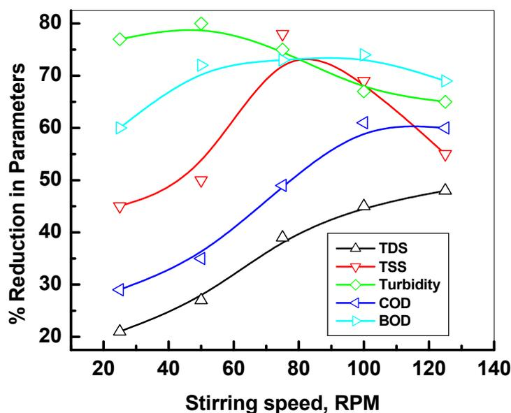
**Figure 9** Effect of variation of stirring speed with parameter reductions.
