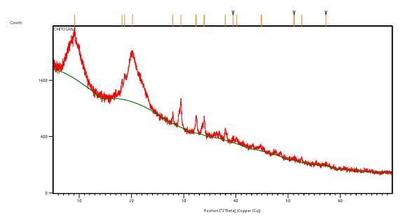
Figure 3 X-Ray Diffraction pattern of chitosan powder.
