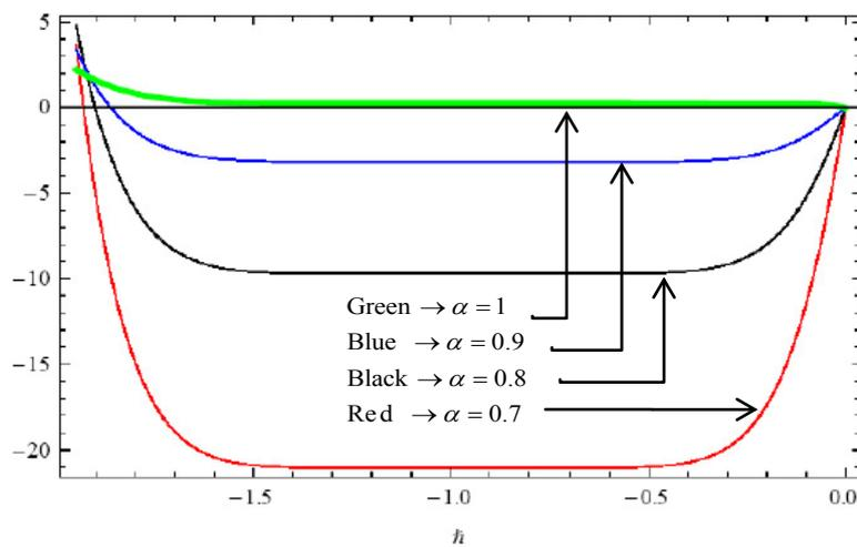
**Figure 2** Plot of the  $\tilde{h}$  curves for different values of  $\alpha = 0.7, 0.8, 0.9$  and 1 for Example 1.
