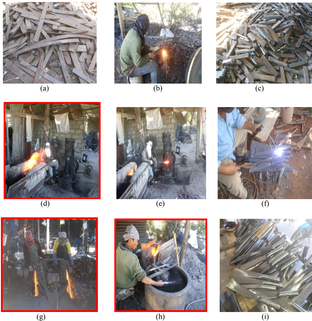
Figure 5 Process of production machetes; (a) Leaf spring steel, (b) Cutting steel with LPG gas, (c) Steel to make the machete (d) Classic furnace, (e) Forging machete with machine, (f) Welding handgrip machete, (g) Grinding, (h) hardening process, (i) The machetes the production.
